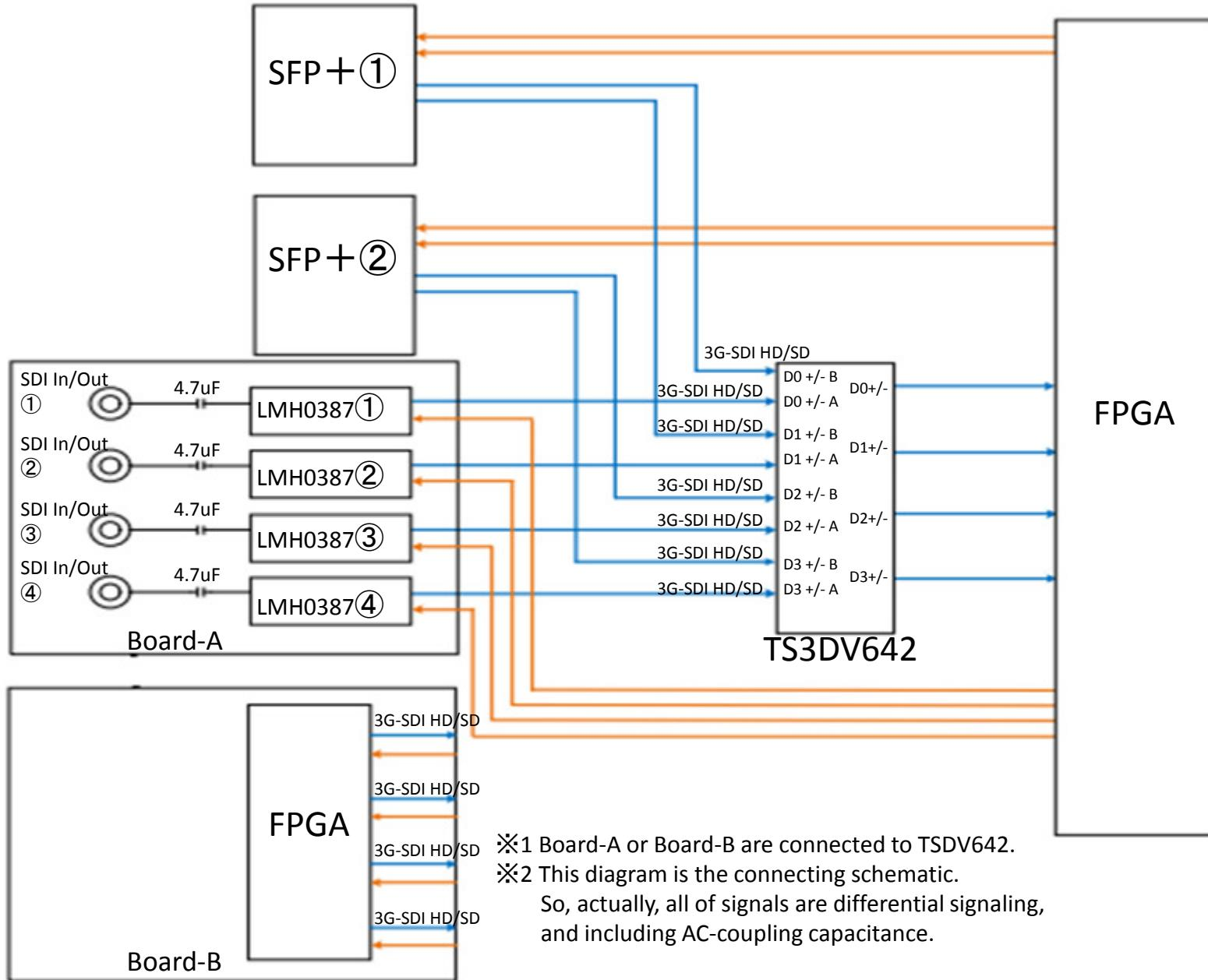
※1 Board-A or Board-B are connected to TSDV642.
