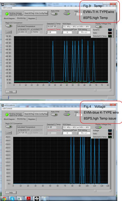
We discovery the high temp curve can be show when dragging the softwave window. We have some experiment with 8SPS 16SPS 32SPS 64SPS 128SPS 250SPS 475SPS \$60SPS. The high temp curve is alway show with 8SPS. The high temp curve is show sometimes with 16SPS \$32SPS. The high temp curve is never show more than 64SPS. I consider maybe the issue source from the ADS1118EVM softwave,but I can't sure it.
