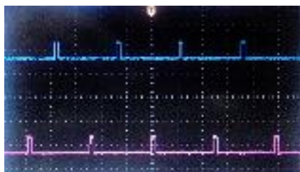
Figure 9: LED Driving Signal coded using MCU and tested on oscilloscope.
