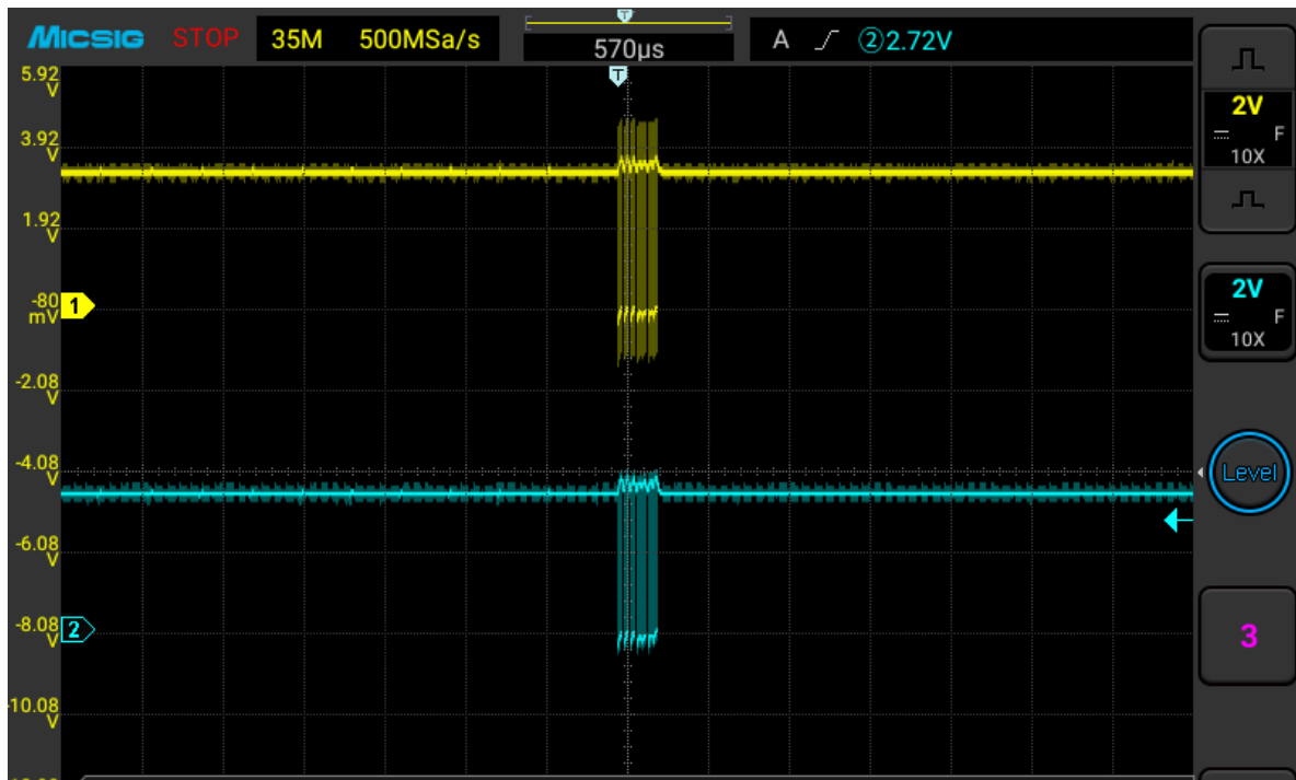
Fig 03: CAN_TX (yellow) & CAN_RX (sky-blue) with 5ms time division
