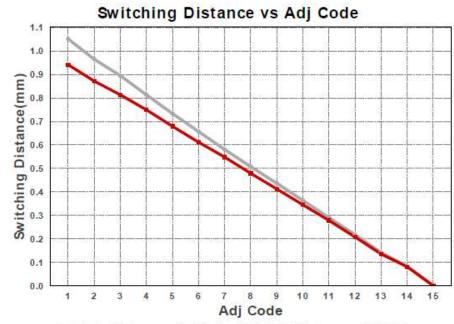
■Switch On Distance vs Adj Code ■Switch Off Distance vs Adj Code
