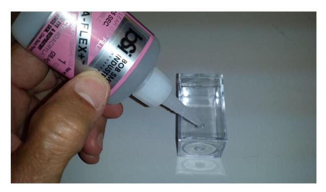
5. Attach transducer to glue spot with leads out to side of container
