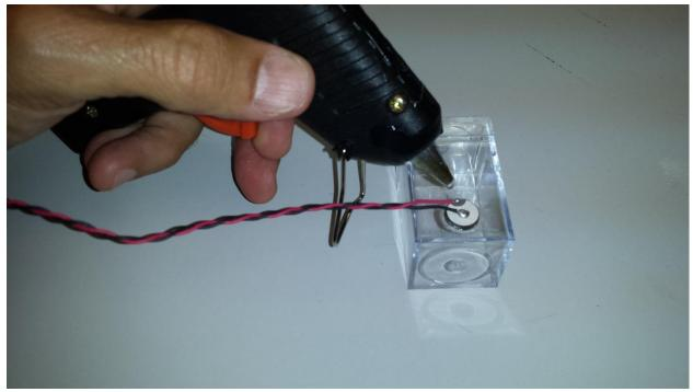
10. and continue covering transducer until it is completely covered in hotglue
