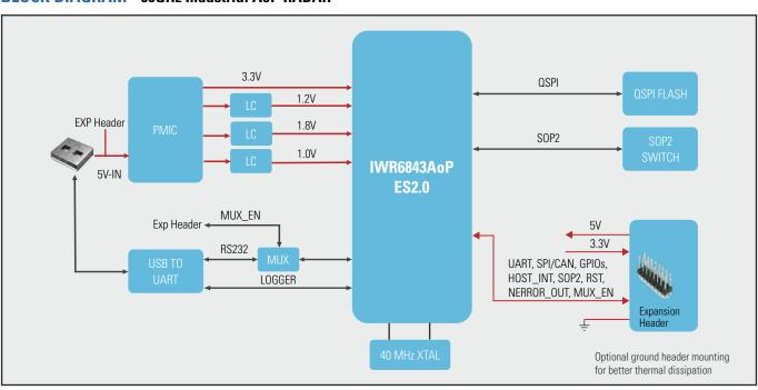
The 60GHz Industrial AoP RADAR is built around IWR6843AoP ES2.0 from Texas Instruments, assuring long lifecycle and support. Mistral adds value by supplying pre-certified AoP RADAR module which helps customer to accelerate time to market, reduce certification risks and ensure seamless product integration.
