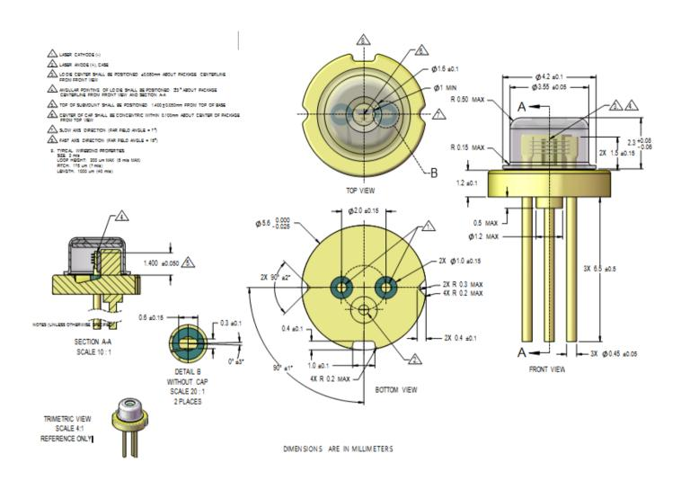
Figure 1. Mechanical Specification
