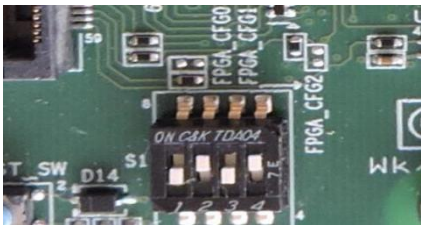
Figure 4: FPGA Config Switch
