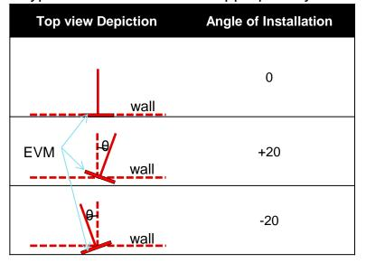
The "scene.azimuthTilt" parameter in the GUI needs to be configured as below
