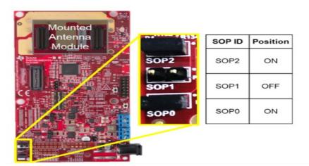
Step 7: Press the Reset for activate flash mode
