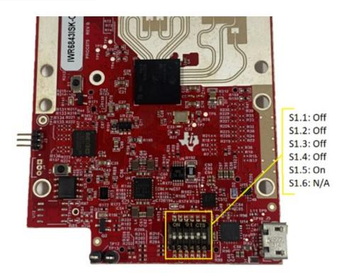
Step 4 : remove the jumper SOP2 Jumper OPEN SOP1 Jumper OPEN SOP0 Jumper CLOSE (edited)
