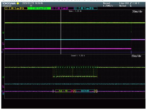
2. Temp and humid data reading out after 100ms wait time
