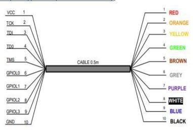
13.1 Connection Table of SPI Interface of xWRL6432 with C232HM-DDHSL-0 Cable
