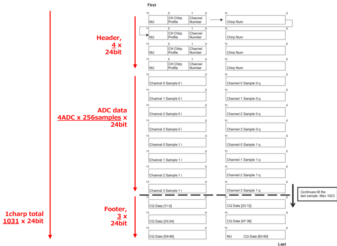
https://www.ti.com/document-viewer/awr2243/datasheet Figure 8-5. Data Packet Packing Format for 12-Bit Complex Configuration
