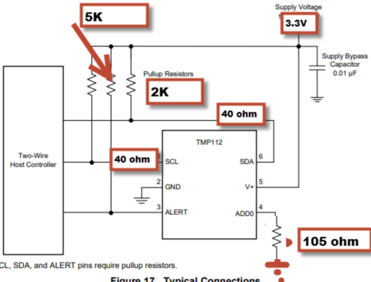
Figure 17. Typical Connections
