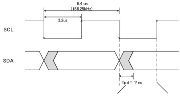
SDA output trigger is SCL falling edge.
