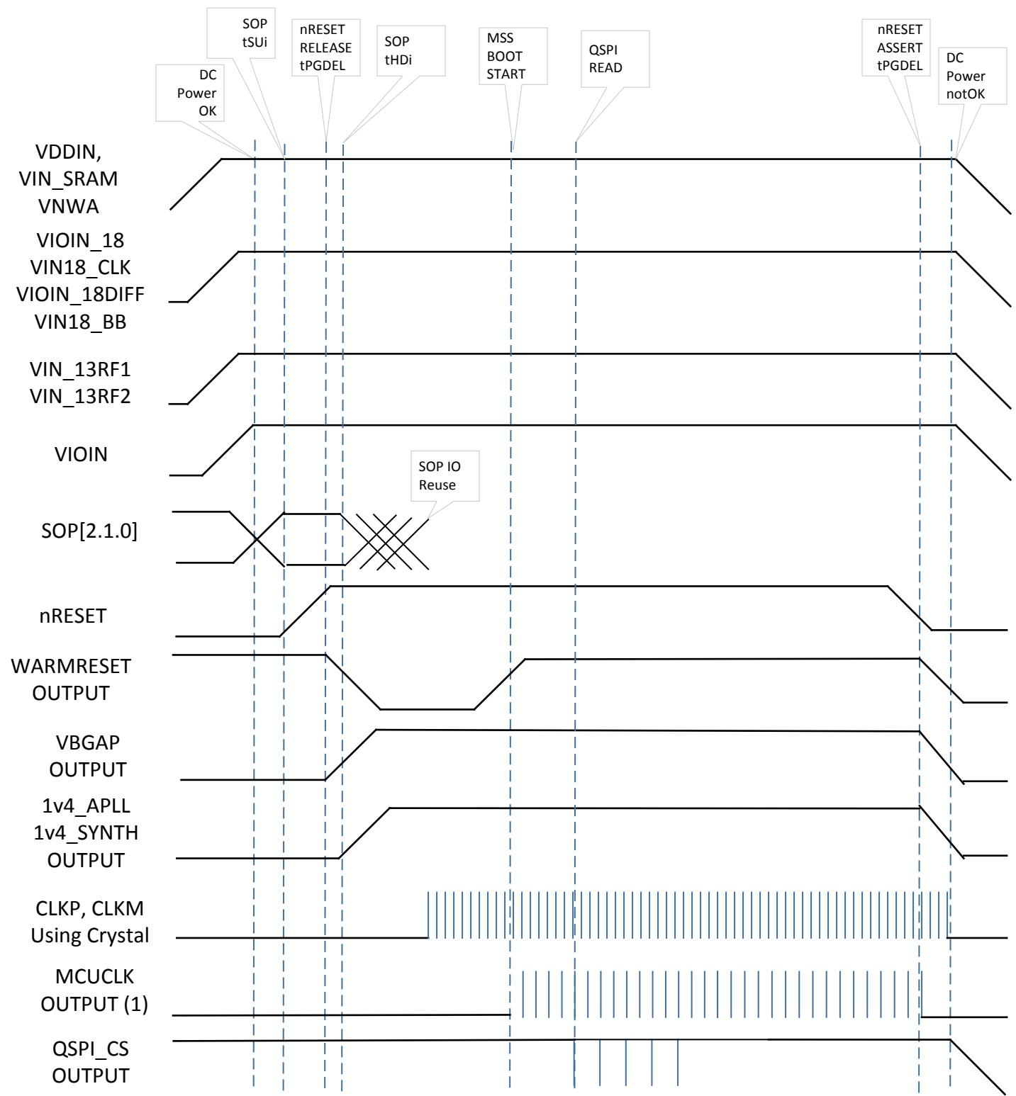
(1) MCU\_CLK\_OUT in autonomous mode, where IWR1443 application is booted from the serial flash, MCU\_CLK\_OUT is not enabled by default by the device bootloader.
