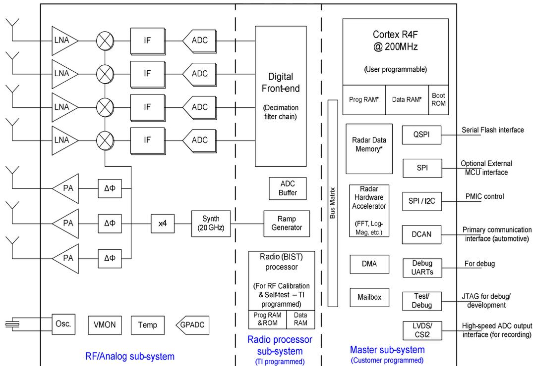
\* Total RAM available in Master sub-system is 576 KB (for Cortex R4F Program RAM, Data RAM and Radar Data Memory)
