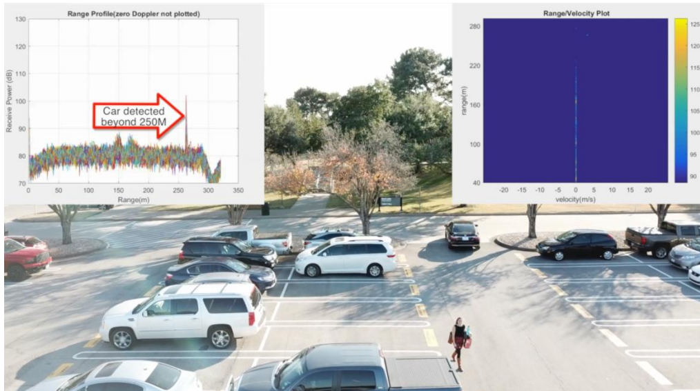
Fig 37: Detection of car beyond 250 meters
