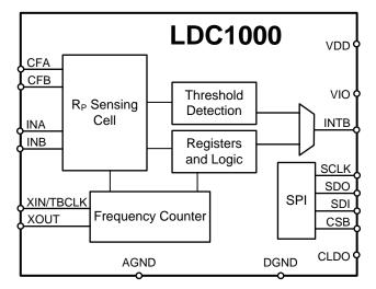
Figure 8. LDC1000 Block Diagram
