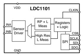
Figure 6. LDC1101 Block Diagram
