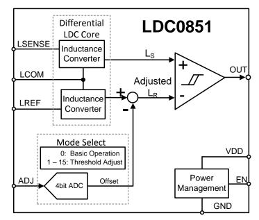
Figure 7. LDC0851 Block Diagram
