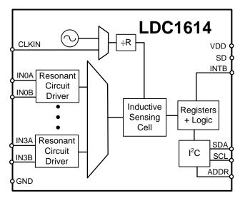
Figure 5. LDC1614 Block Diagram
