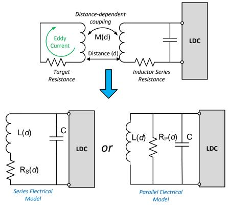
Figure 3. Electrical Model of Parallel Inductive Sensor
