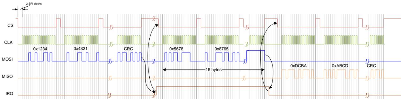
**Figure 5-5. SPI Communication**
