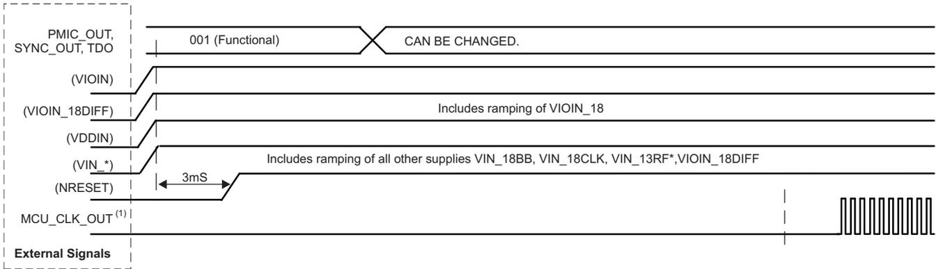
(1) MCU\_CLK\_OUT in autonomous mode, where AWR1243 application is booted from the serial flash, MCU\_CLK\_OUT is not enabled by default by the device bootloader.
