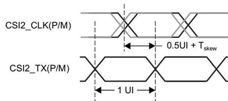
**Figure 5-6. Clock and Data Timing in HS Transmission**
