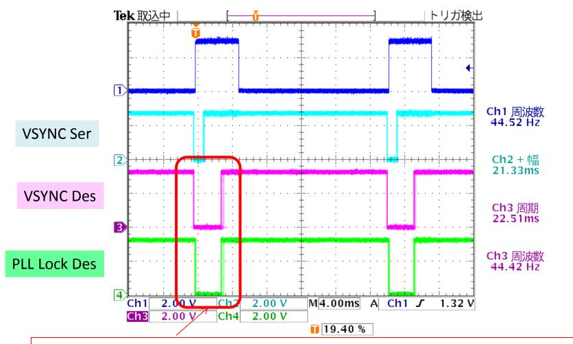
VSYNC Des low output is longer than VSYNC Ser and this time is synchronized with PLL lock output of Des.
