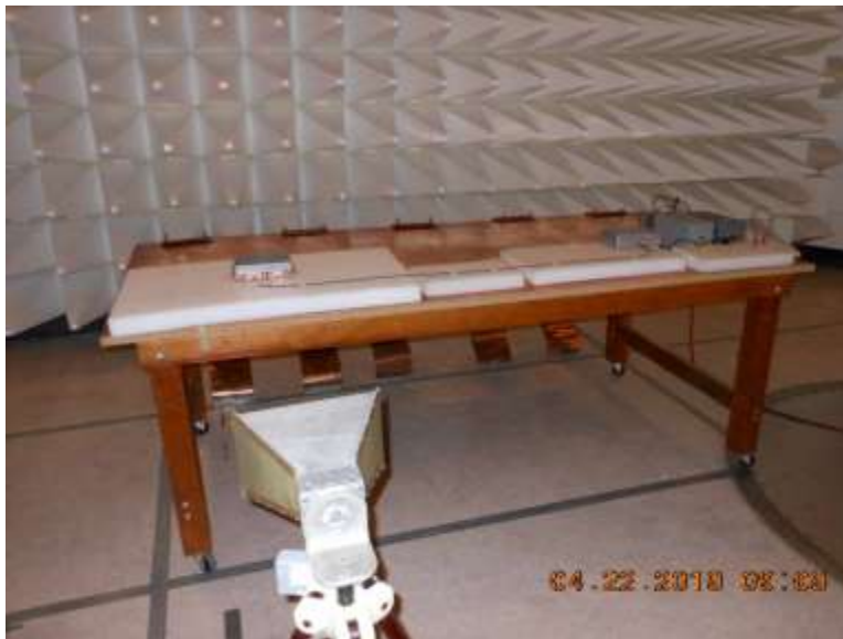
Ambient, HF Horn Antenna, 1-3GHz, Vertical Polarization
