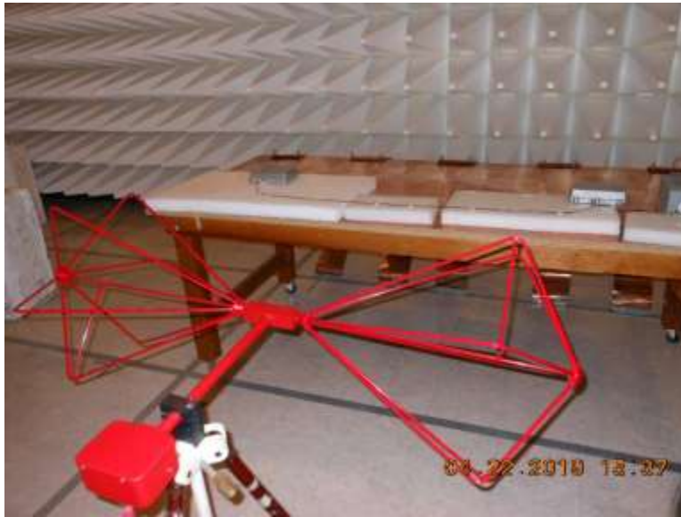
Ambient, Bicon Antenna, 30-200MHz, Horizontal Polarization
