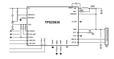
Buck provides ILIMIT & Short to Battery protection.
