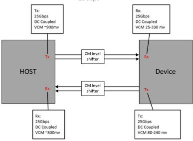
UFS Device is DC couple device with next parameters:
