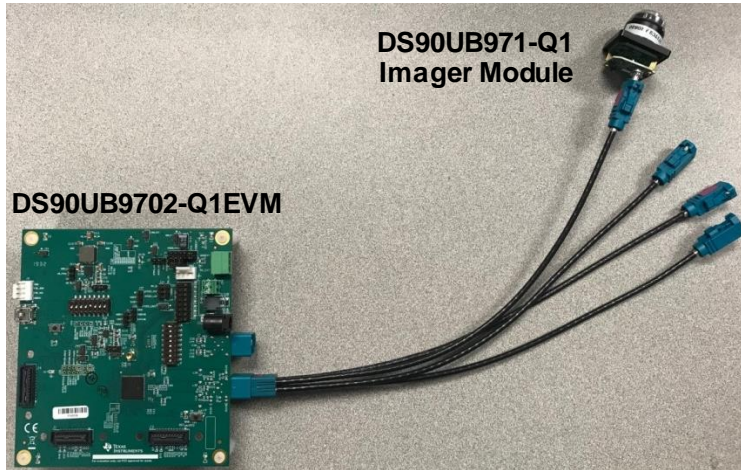
Figure 11 V_{PoC} Noise Test Setup
