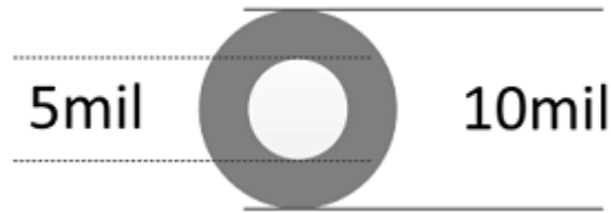
Figure 89. Under Ball Recommended Via Size
