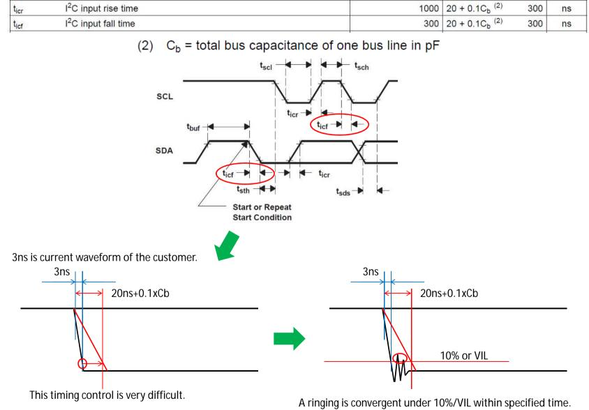
A ringing is convergent under 10%/VIL within specified time Is this waveform OK?
