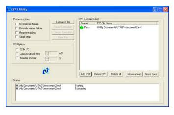
Figure 8-2. Screen Shot of the SCANEase Software indicating that the Board Self-Test Passed
