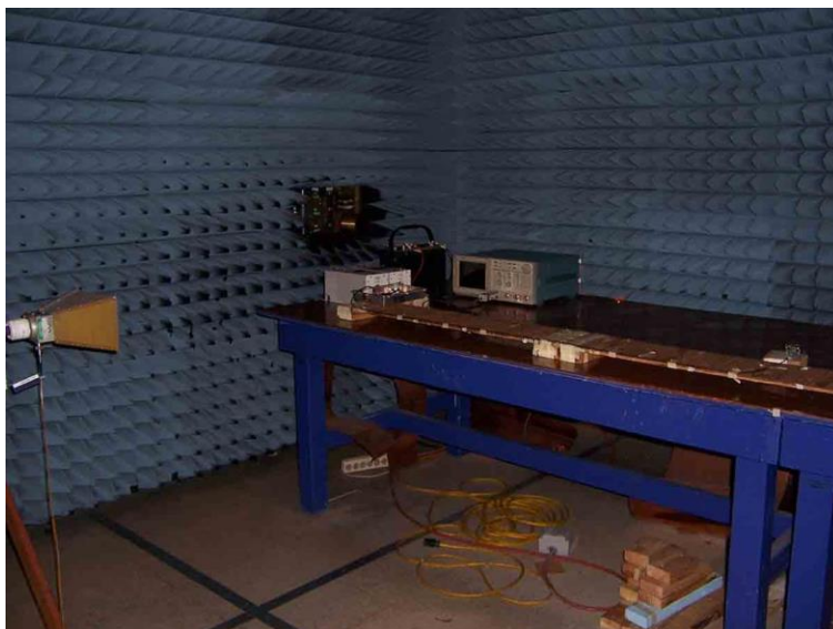
6.4 - 1.567-1.583GHz, HF Horn Antenna, Vertical Polarization, GPS Mobile P1
