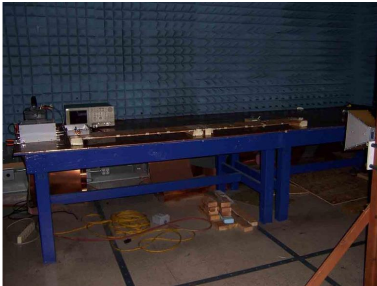
6.4 - 1-2.5GHz, HF Horn Antenna, Horizontal Polarization, Mobile P2
