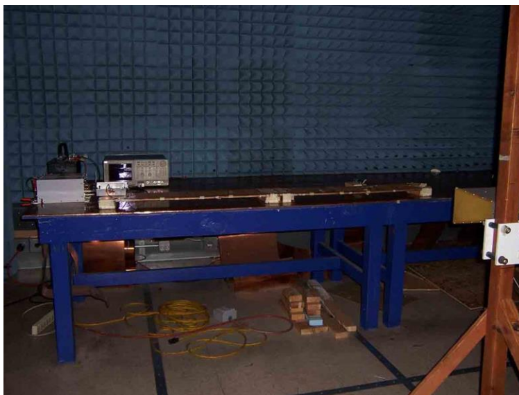
6.4 - 1-2.5GHz, HF Horn Antenna, Vertical Polarization, Mobile P2
