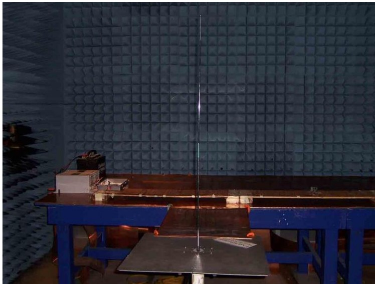
6.4 - 26-30MHz, Rod Antenna, Vertical Polarization, Mobile
