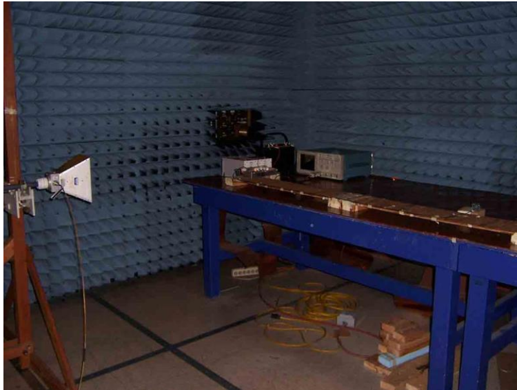
6.4 - 1-2.345GHz, HF Horn Antenna, Horizontal Polarization, Broadcast P1
