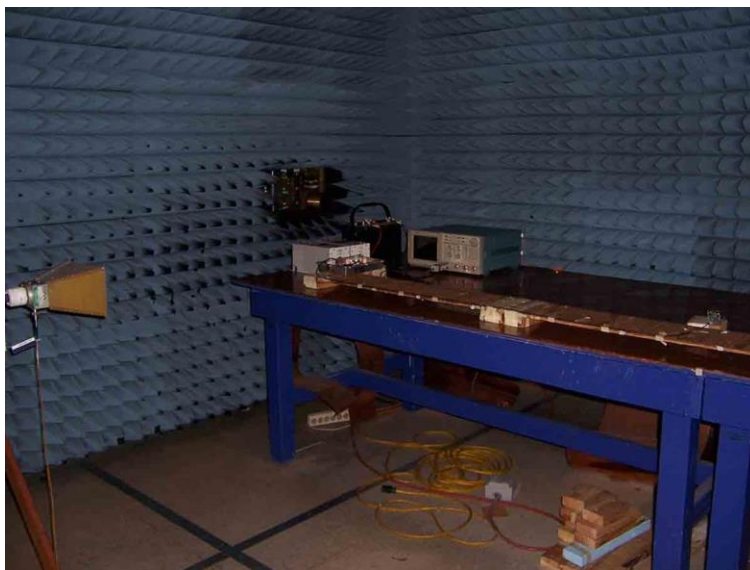
6.4 - 1-2.345GHz, HF Horn Antenna, Vertical Polarization, Broadcast P1
