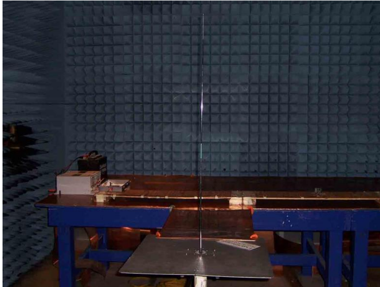
6.4 - 0.15-30MHz, Rod Antenna, Vertical Polarization, Broadcast
