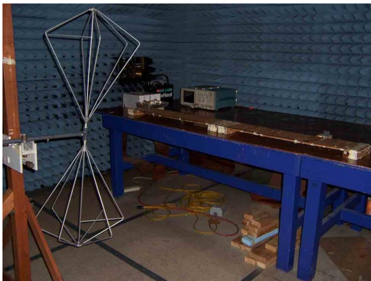
6.4 - 30-300MHz, Bicon Antenna, Vertical Polarization, Broadcast
