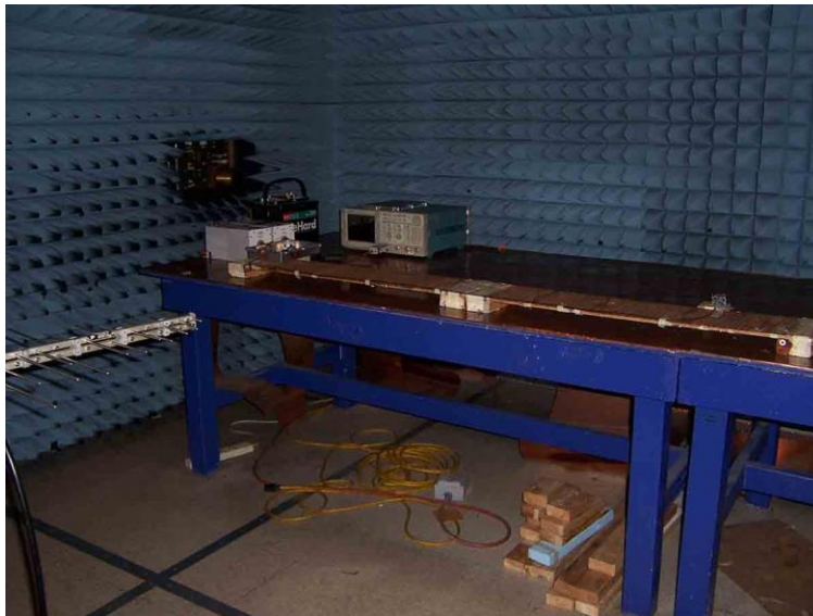
6.4 - 300MHz-1GHz, Log Antenna, Horizontal Polarization, Mobile
