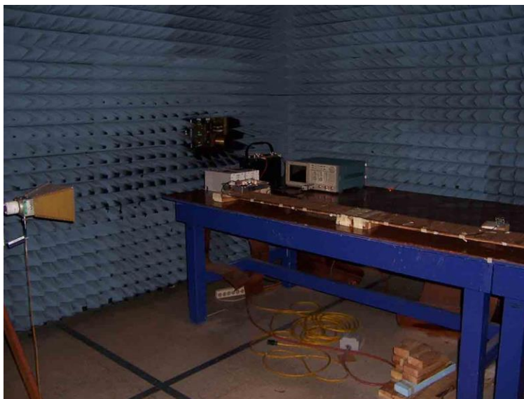
6.4 - 1-2.5GHz, HF Horn Antenna, Vertical Polarization, Mobile P1
