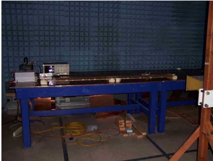
6.4 - 1.567-1.583GHz, HF Horn Antenna, Vertical Polarization, GPS Mobile P2
