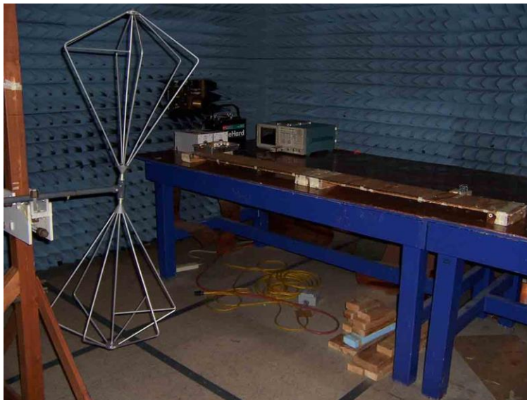
6.4 - 30-300MHz, Bicon Antenna, Vertical Polarization, Mobile
