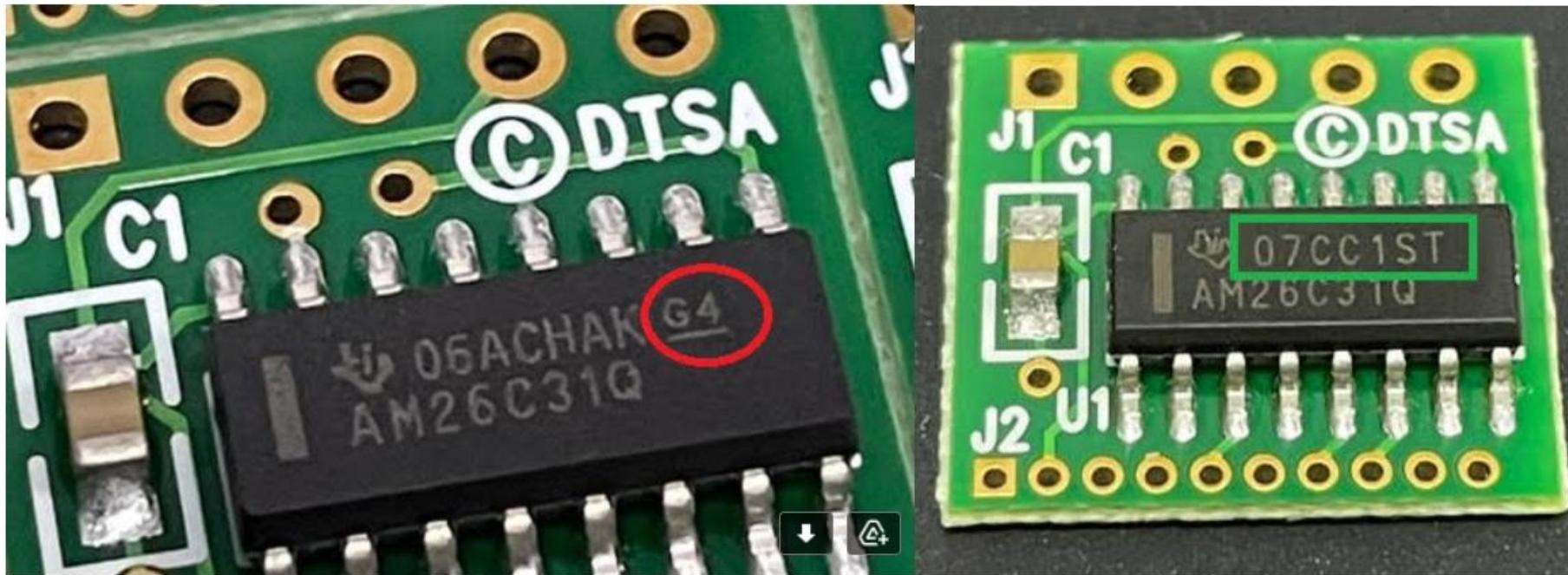
(Good part) AM26C31Q lead finish - CU NIPDAU & CU SN
