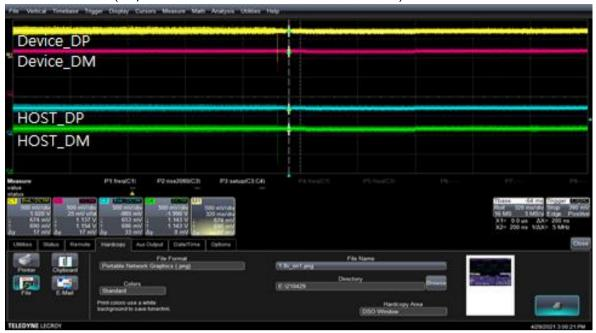
2. Normal status (DP/DM waveform of device and host side)
