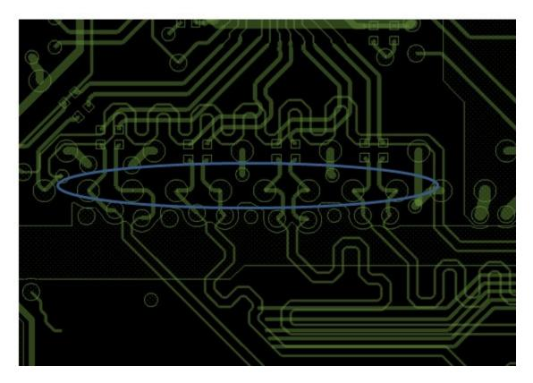
Second thing I noticed is the inter-pair skew on the DSI interface. The DSI86 samples data on rising and falling edge of DSI clock. Any variation in length between CLK and DATA lanes will impact setup and hold requirement. My recommendation is to match lane length as close to each as possible. DSI\_A data/clock should be within 5 mils of each other.
