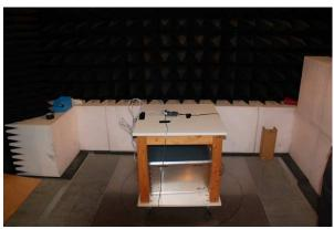
Figure 59. Automatic Pre-Test Setup for EMI With 3-m Antenna Distance to DuT (Left: Antenna, Right: TIDA-00204 DuT and Box With Shielded Laptops)
