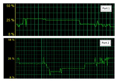
Figure 63. IEC61000-4-2 ±6-kV ESD CD: Network Utilization With UDP Packet Throughput Test on Port 1 and Port 2 (Measured on Two Separate Laptops)
