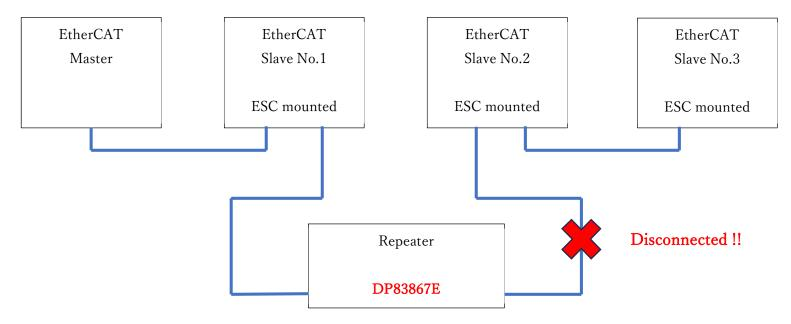
In an EtherCAT network, I would like to connect the DP83867E back-to-back to function as a repeater and insert it as an infrastructure component in the network.
