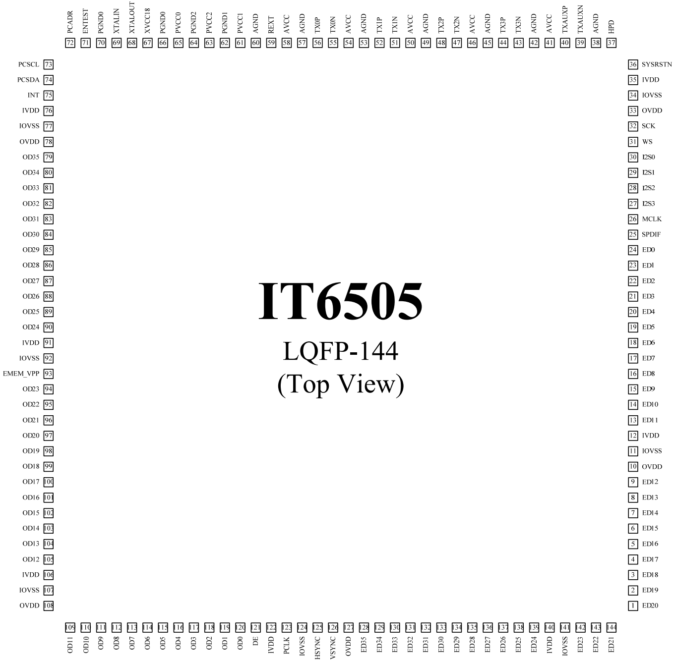
Figure 1. IT6505 pin diagram
