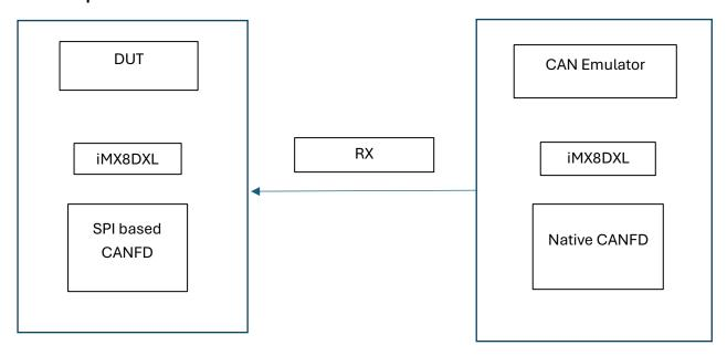
The SPI frequency is set to **16 MHz**, and the **watermark level** for the m\_can driver is configured to **26**, which triggers an interrupt after 26 messages are received. Upon interrupt, the SPI transfer for receiving messages starts.
