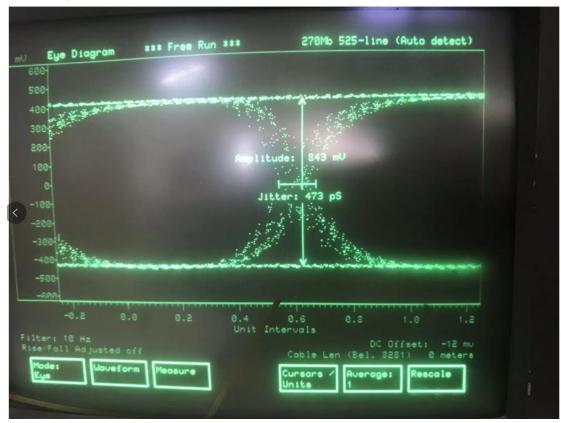
(6) At last,we removed the failed port's LMH0397 and soldered a new one,then this port works good.
