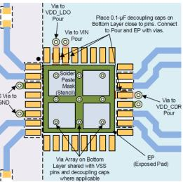
Top solder paste: Please follow LMH1297 data sheet figure 42 – high speed trace layout recommendations.
