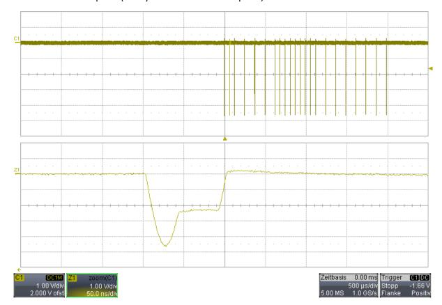
External Loopback with 50 cm CAT6 cable and loopback connector (pin 1 to 3 and pin 2 to 6) – continuous signal changes:
