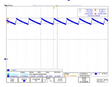
V-  $0.047\mu F$  C1 and  $0.047\mu F$  C2 Added  $3k\Omega$  load during measurement
