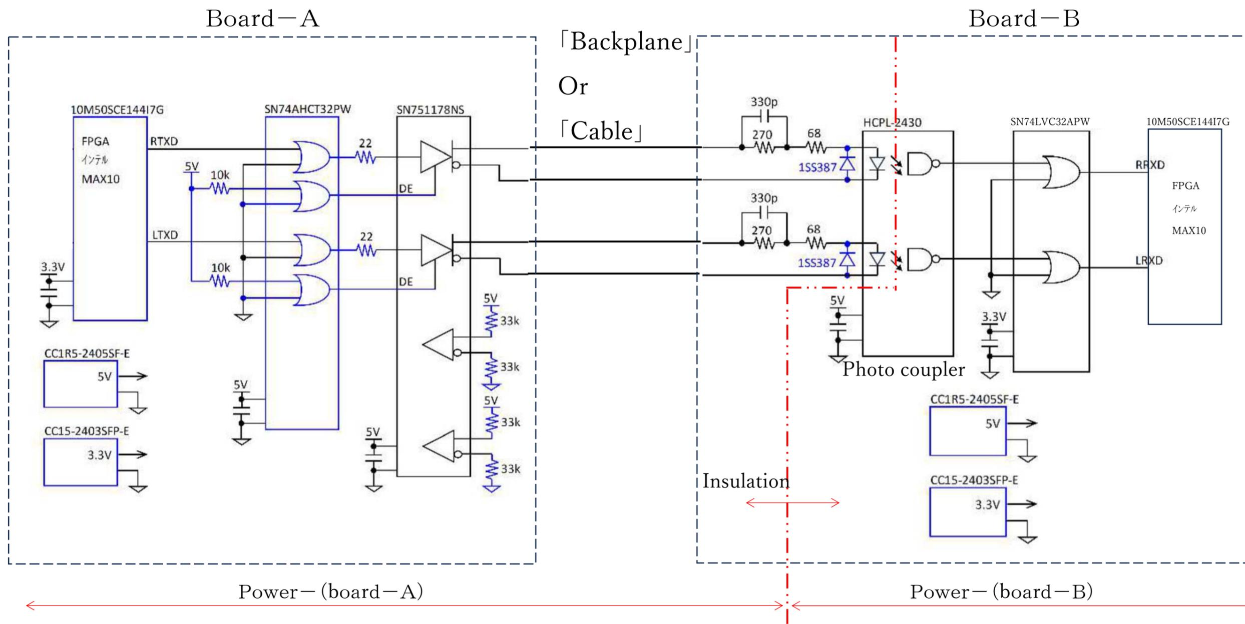
※In the case of backplane connection, the GND of board-A and board-B are not connected.
