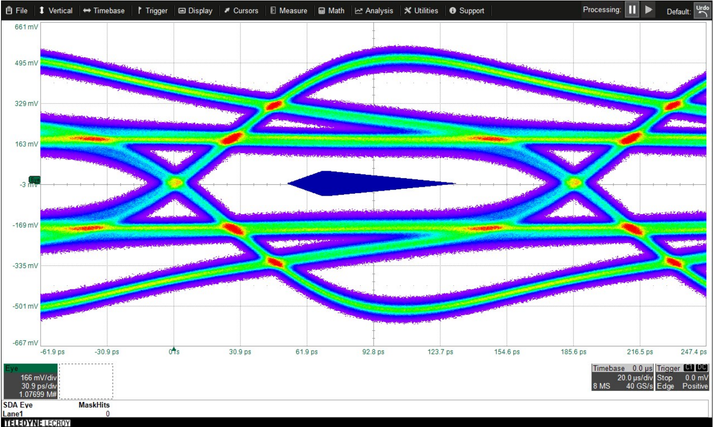
Test 3.1 - TP3_EQ Eye Diagram, Zero Length Lane0 SSC Disabled 5.4 Gb/s Timestamp: 12/24/2019 04:19:29
