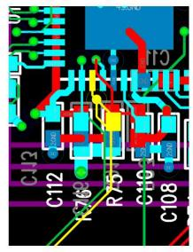
SDA from top layer, down to layer 8. layer 8 is adjacent to a gnd plane.
