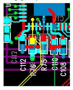
SCL from top layer, down to layer 3. layer 3 is adjacent to a gnd plane.
