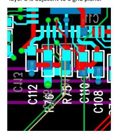
Both route to a pins on a high speed differential connector --- transfers to pins on bottom layer:
