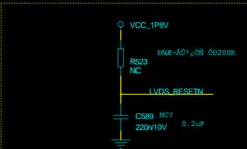
Reset(EN) can be implemented with passive components as shown or active circuitry. In case of using passive components, the values of the RC circuitry need to be adjusted to make sure the low to high transition occurs after the Vcc supply has reached the minimum recommended operating voltage. For this reason, it is recommended to USE ACTIVE CIRCUITRY for better control of the RESET/EN timing.
