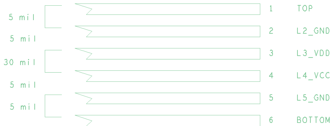
Figure 26. EVM Layer Stack-up
