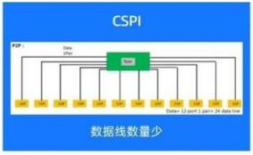
▲ The CSPI protocol can reduce the number of cables by 70%
