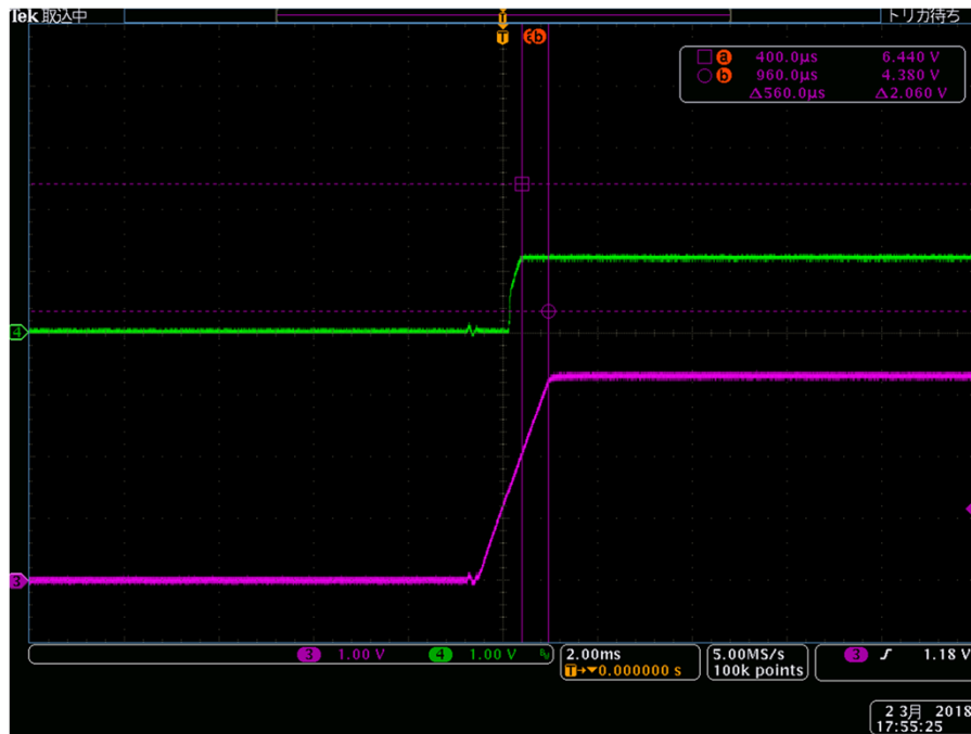
Fig1. TMDs181 EVM Power-up timing
