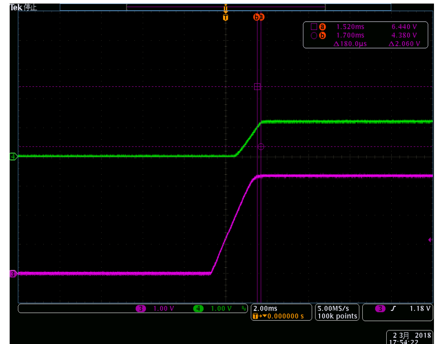
Fig2. Our TMDs 181 board Power-up timing
