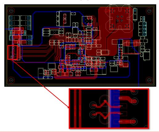
Keep the use of bends in differential traces to a minimum. When bends are used, the number of left and right bends must be as equal as possible, and the angle of the bend should be ≥ 135 degrees.
