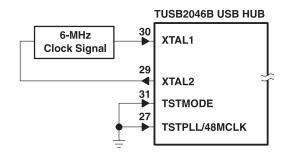
Figure 7. 6-MHz Input Clock Configuration
