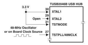
Figure 8. 48-MHz Input Clock Configuration
