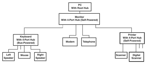
Figure 5. USB-Tiered Configuration Example
