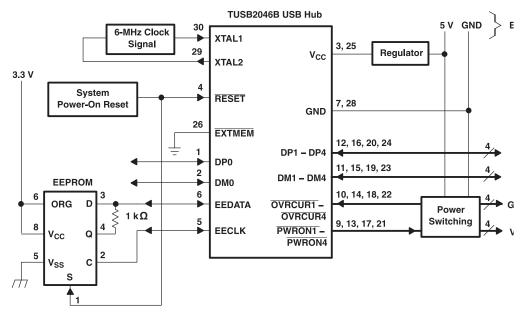
Figure 9. Typical Application of the TUSB2046B USB Hub
