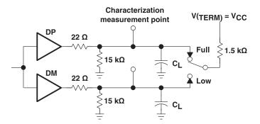
Figure 1. Differential Driver Switching Load
