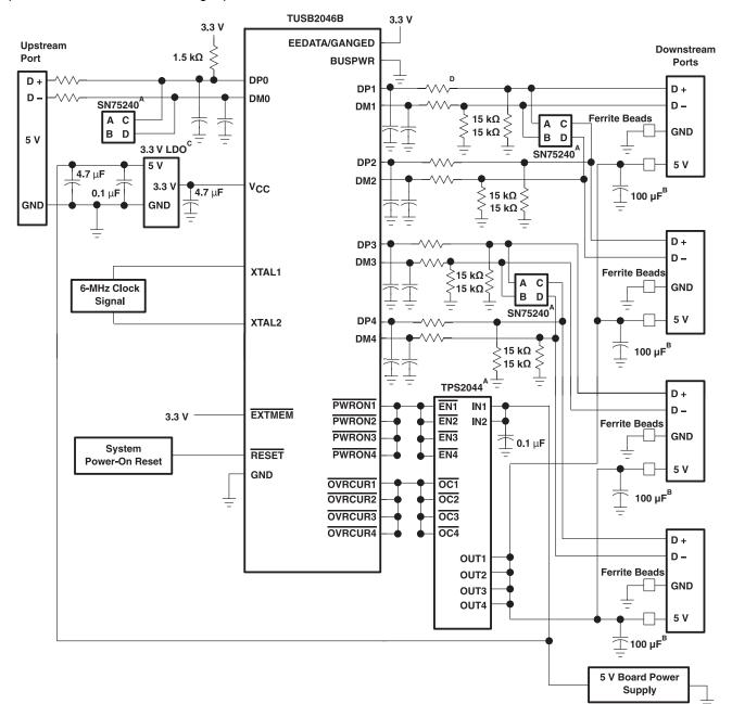
NOTES: A. TPS2044, TPS2042, and SN75240 are Texas Instruments devices. The TPS2042 can be substituted for the TPS2044. The OCn outputs of the TPS204n are open drain. A 10-kΩ pullup is recommended.
